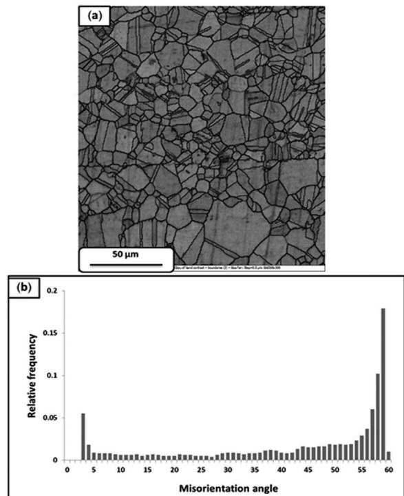
Fig. 4. EBSD Analysis of the coarse grain sample (a) boundaries Map and (b) Misorientation angle distribution.
