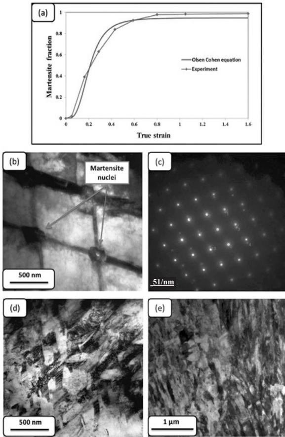
Fig. 2. Martensite area fraction versus true strain during cold rolling (a), TEM micrograph and related SADP of the rolled samples after (b and c) 5%, (d) 35%, and (e) 60 % reduction.
