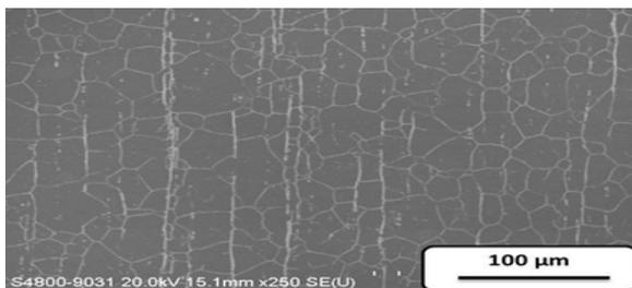
Fig.1. SEM micrograph of the as-received 304L stainless steel.
