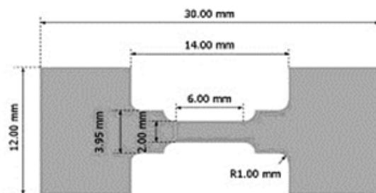
Fig. 1. The geometry of the tensile test specimen.
