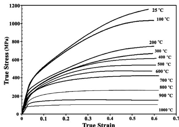
Fig. 1. The effect of hot compression on true stress–true strain response of the hot-rolled specimen.
