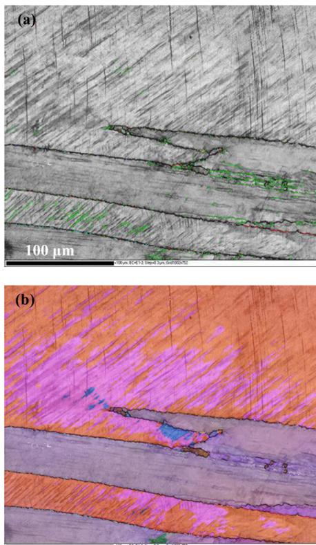
Fig. 4. SEM-EBSD micrographs of the homogenized materials after hot compression at 900°C to 0.6 true strain under strain rate of 0.01 s<sup>-1</sup>: (a) band contrast image and (b) color map. The green lines represent the moderate misoriented deformation twin with angle of 15°.
