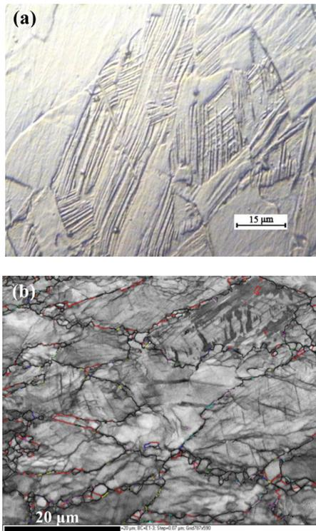
Fig. 3. The microstructure of hot-rolled specimen after straining to 0.6 at 800°C: (a) optical micrograph and (b) SEM-EBSD (band contrast) micrograph.
