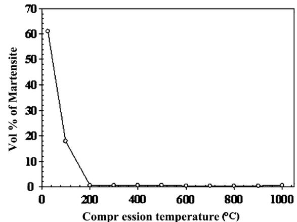
Fig. 2. The effects of compression temperature on deformation-induced martensite formation.
